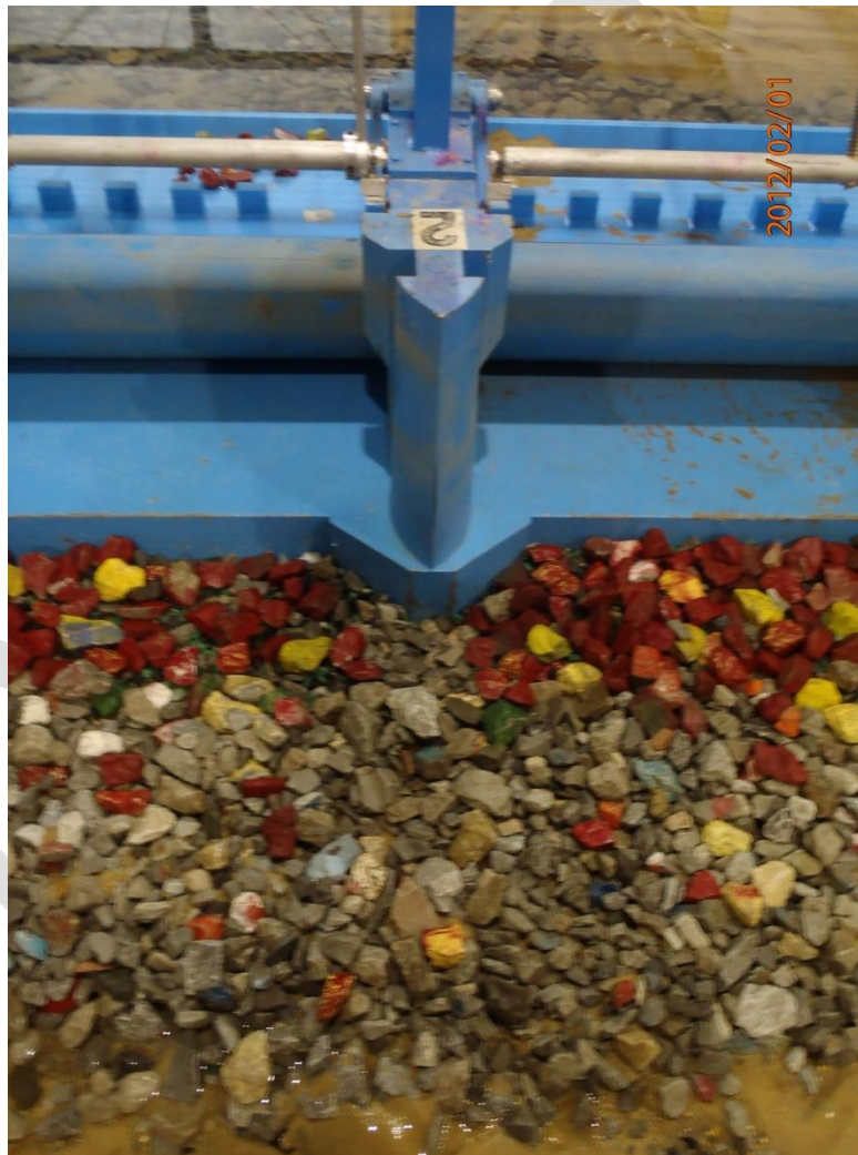
Figure 12 - 9 ft center gates, modified “A” stone over modified “C” stone
