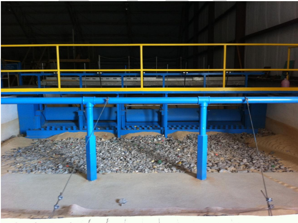
Figure 4 - The model gate structure and walkway viewed from downstream
