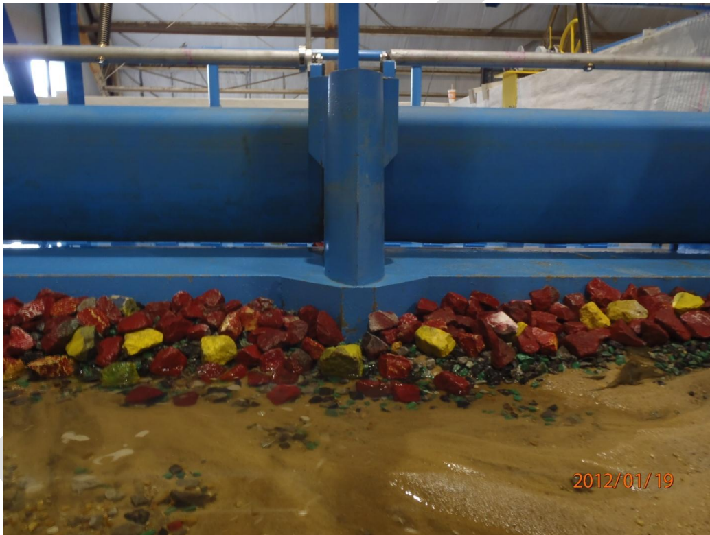
Figure 10 - 7 ft center gates, 20 ft ice raft draft
