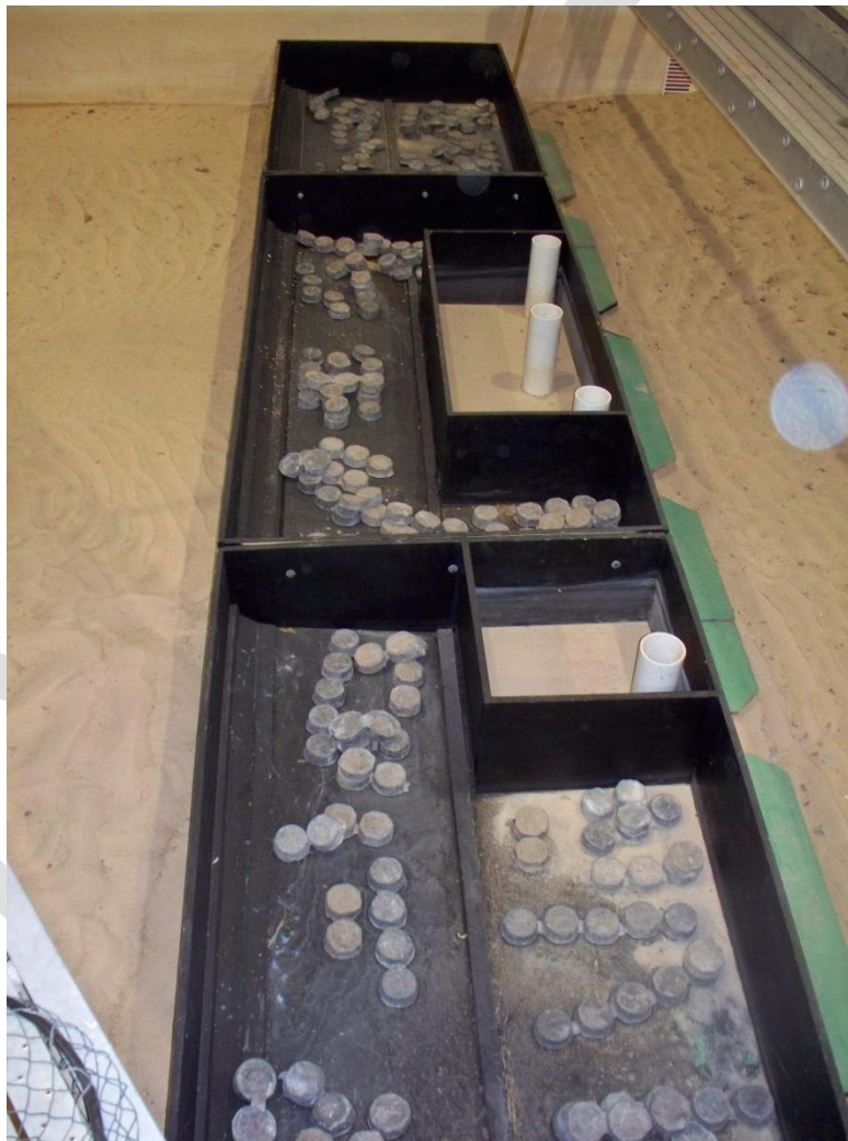
Figure 5 - Wooden raft used to simulate upstream ice
