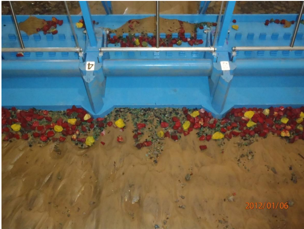
Figure 8 - Variable 3 center gates, 15 ft ice raft draft
