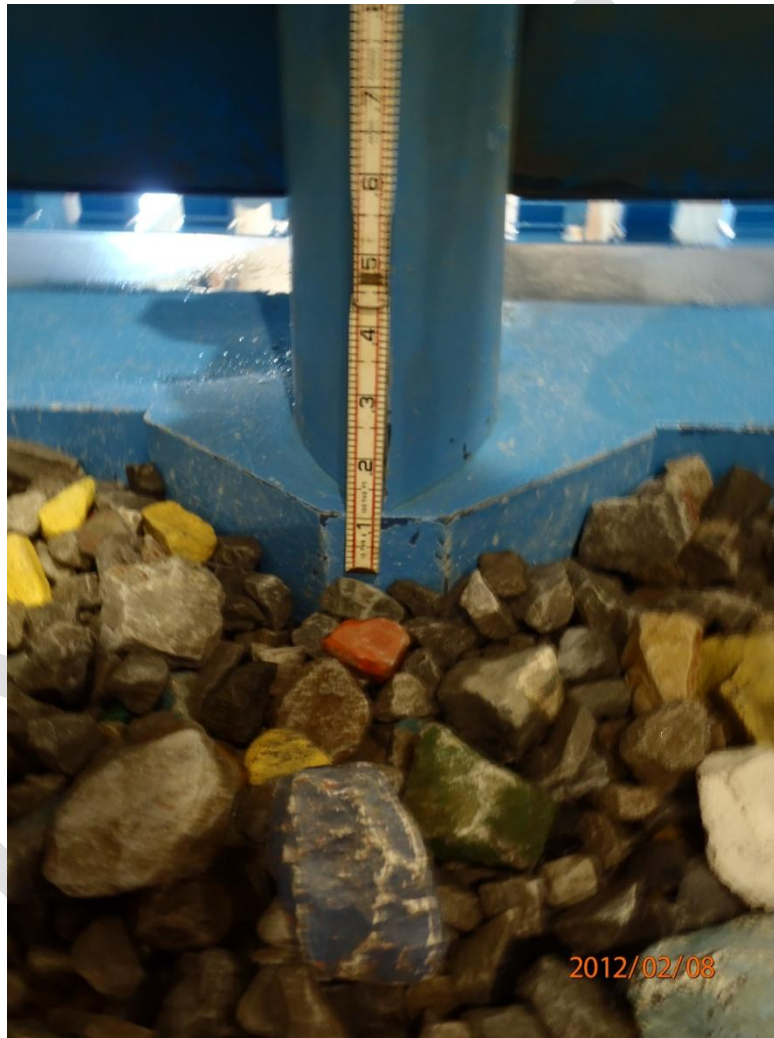
Figure 14 - 9 ft center gates, 5 ft side gates, modified "A" stone over modified "C" stone
