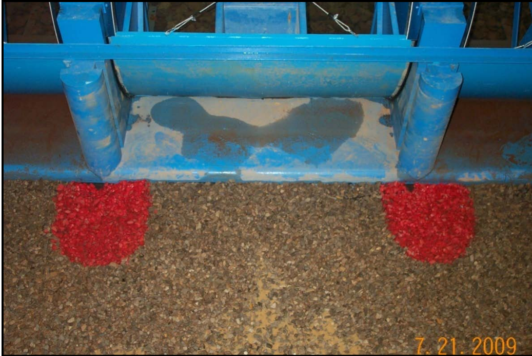
Figure 10 - Post-test conditions for a 23 ft. center gate opening Upper pool = 419 ft., original stone placement test
