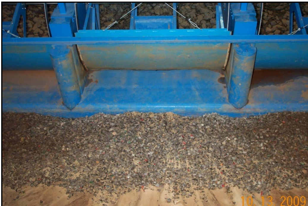
Figure 14 - 23 ft center gate opening, original stone, no filter cloth, with ice raft
