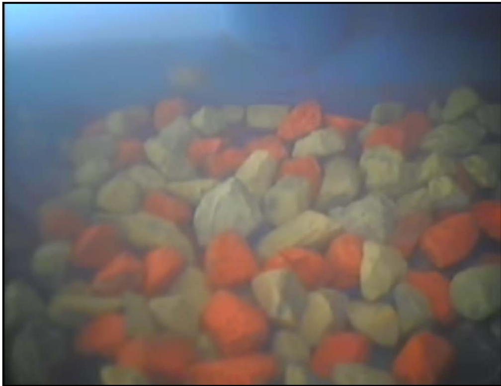
Figure 26 - Orange and yellow stone cap layer movement
