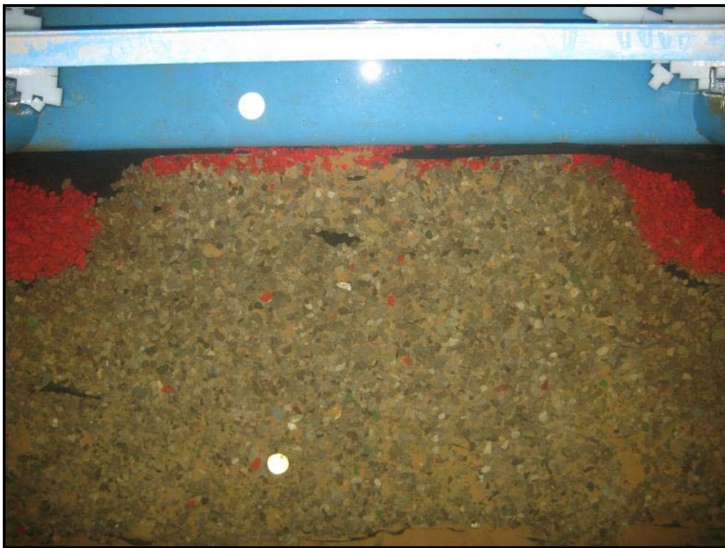
Figure 18 - Pier Scour after testing with a 13 - 14 ft ice raft draft
