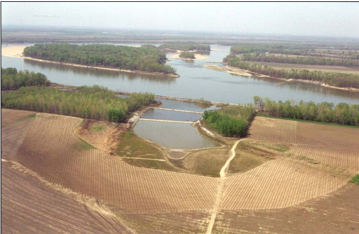
Figure 78: Tree Screens and Rock Baffles for Overbank Scour Protection at Dry Bayou on the Mississippi River (Rapp 2005)
