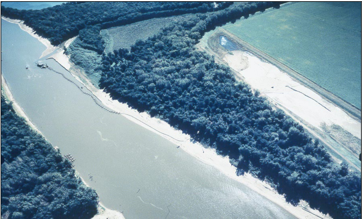
Figure 20: Dredging and Off-Channel Disposal on the Illinois River (Cox 2005)
