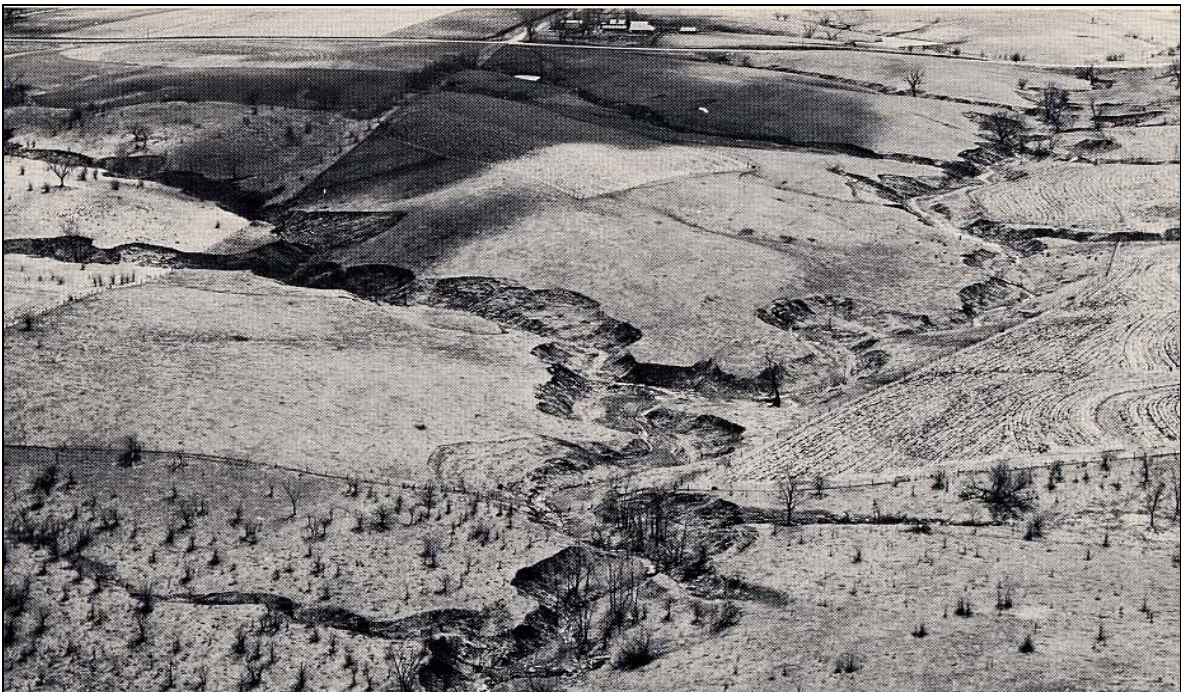
Figure 7: Channel Degradation (Downcutting or Headcutting) on a Small Stream in Iowa
