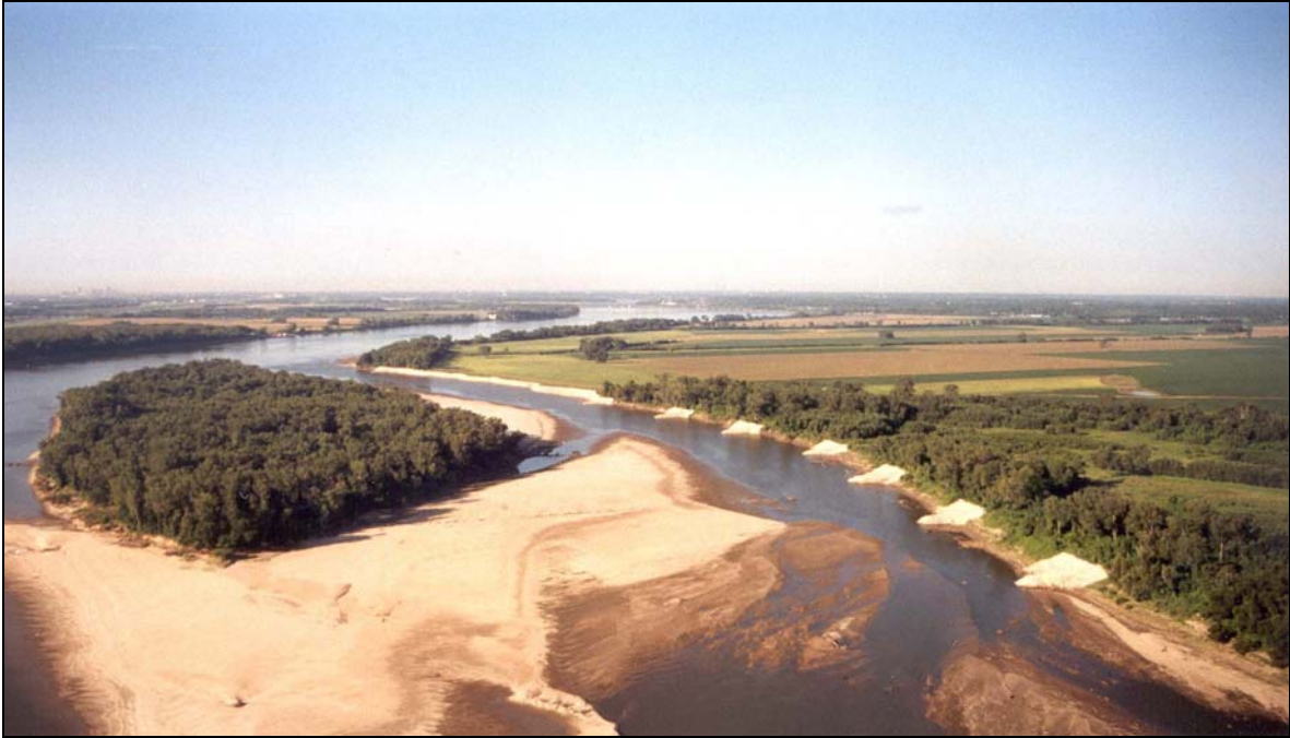
Figure 80: Hardpoints for Bank Protection in a Side Channel of the Middle Mississippi River (Hopkins 2005)
