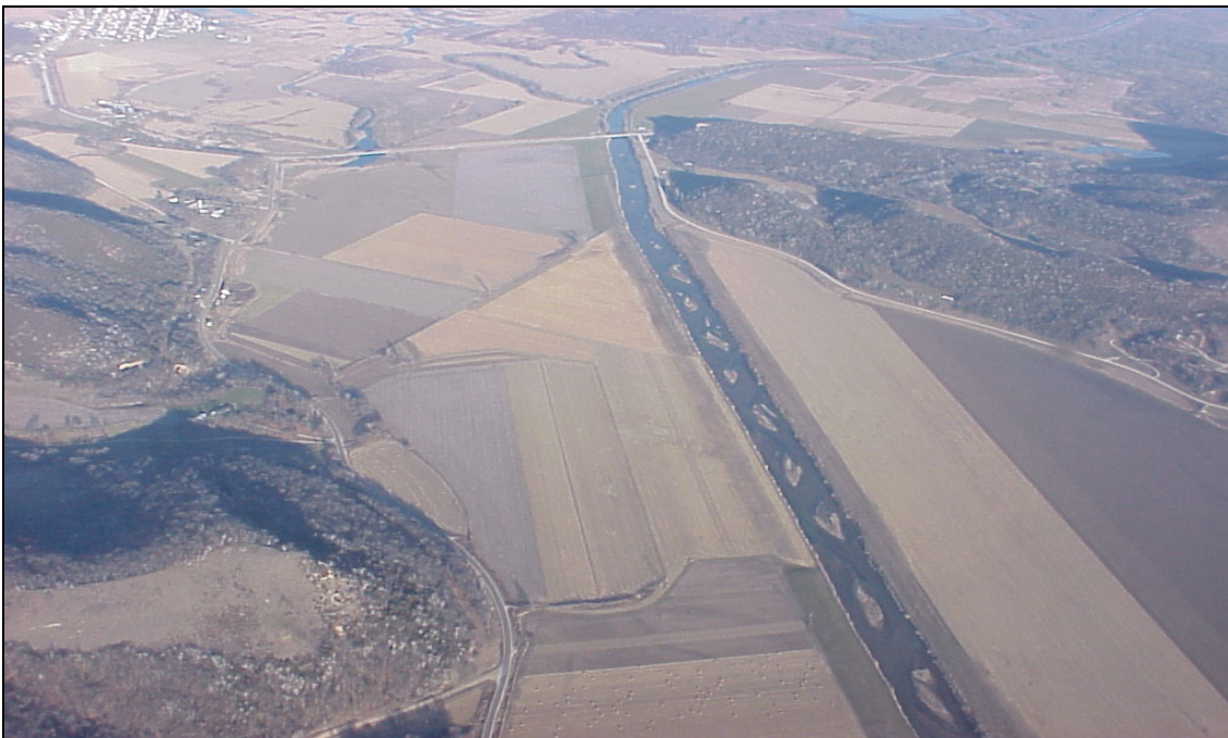
Figure 11: Sedimentation and New Meander Pattern Established in Channelized Portion of the Upper Iowa River
