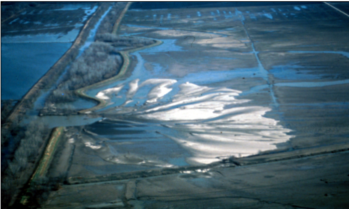
Figure 13: Concentrated Sand Deposit over the Floodplain after a Levee Breach on Bryants Creek, Missouri. near the Mississippi River at Mile 200
