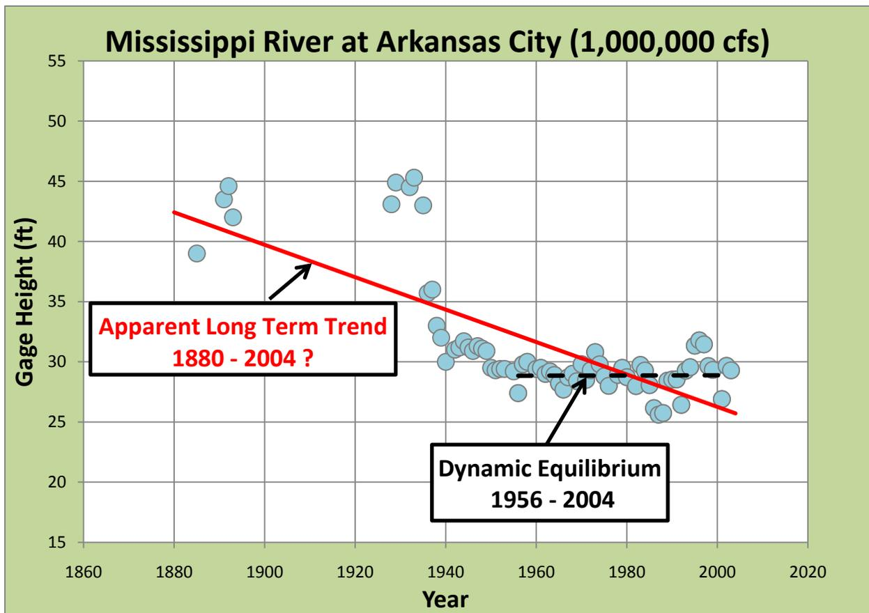
**Figure 3.1** The specific gage record for the Mississippi River at Arkansas City for the period 1880 to 2004 for a flow of 1,000,000 cfs.
