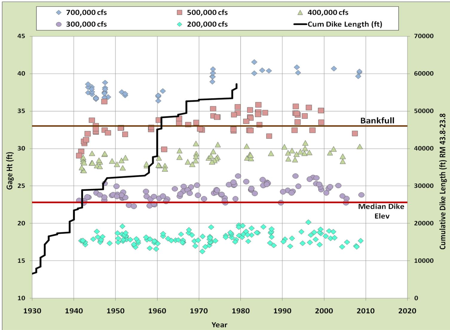
Figure 5.3 Specific gage record for the Thebes gage for the period 1941 to 2009.
