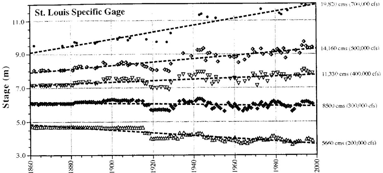
**Figure 4.1** The specific gage graph was suggested by Pinter et al. (2001) to show apparent trends in stage through time.
