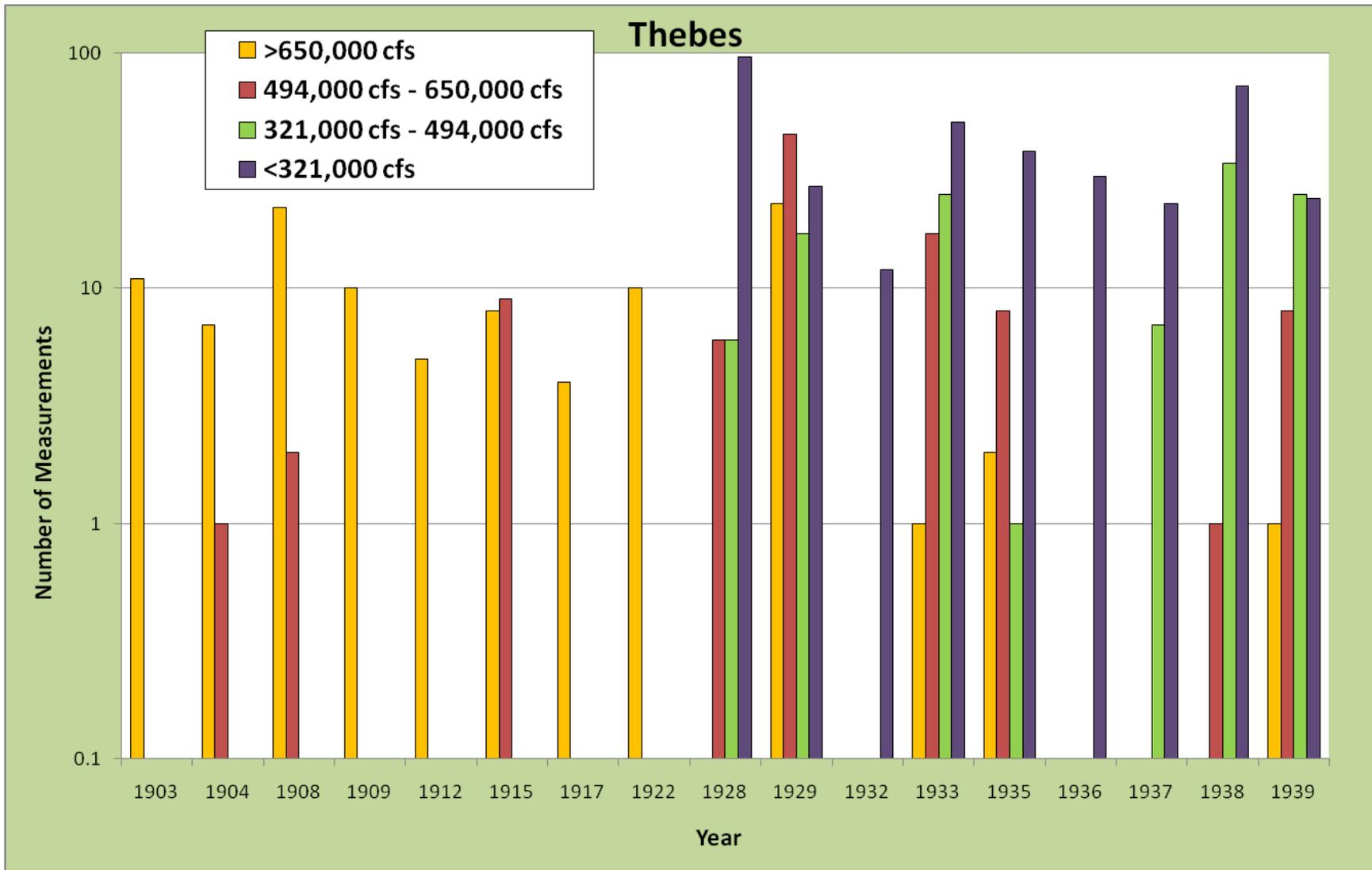
Figure 4.7 The number of measurements made in four discharge ranges at Thebes from 1903 to 1939.
