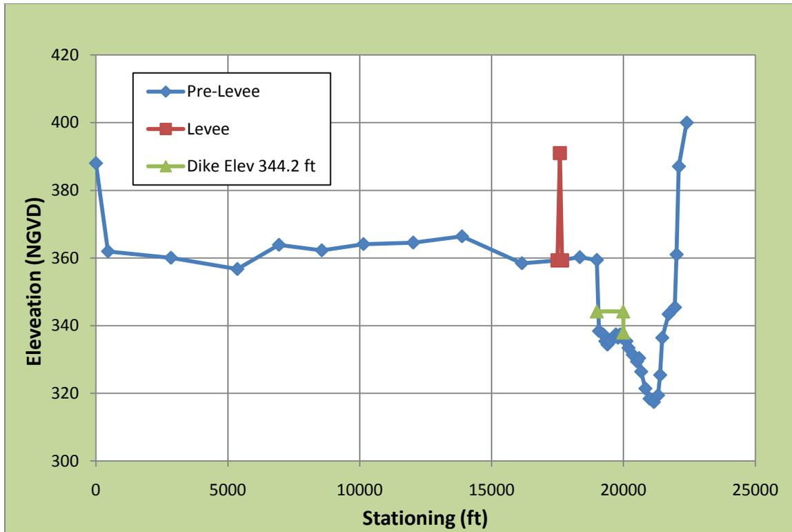
Figure 5.4 Valley cross section near RM 103.5 downstream of Chester IL
