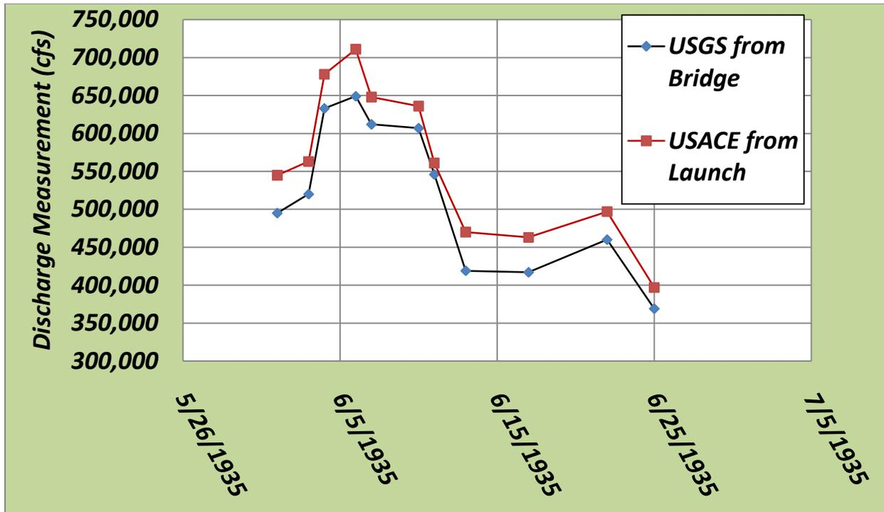
**Figure 4.8** The graph displays the data collected in 1935 during simultaneous measurements using USGS and USACE meters. Note that the USACE equipment consistently over-estimated the USGS measurement.
