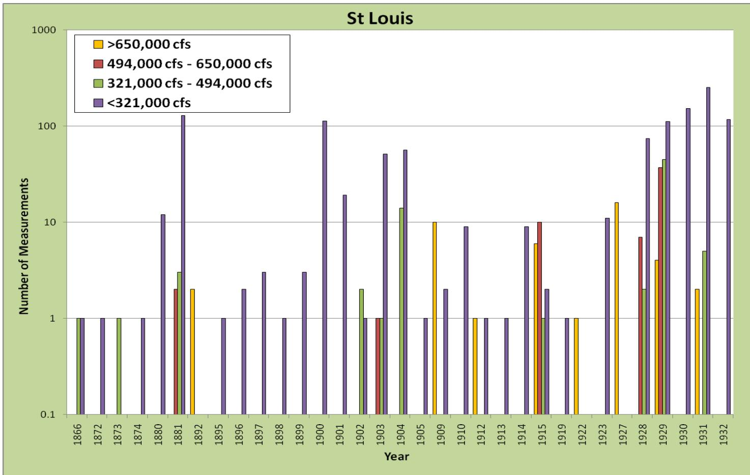
Figure 4.3 The number of measurements made in four discharge ranges at St Louis from 1866 to 1932.
