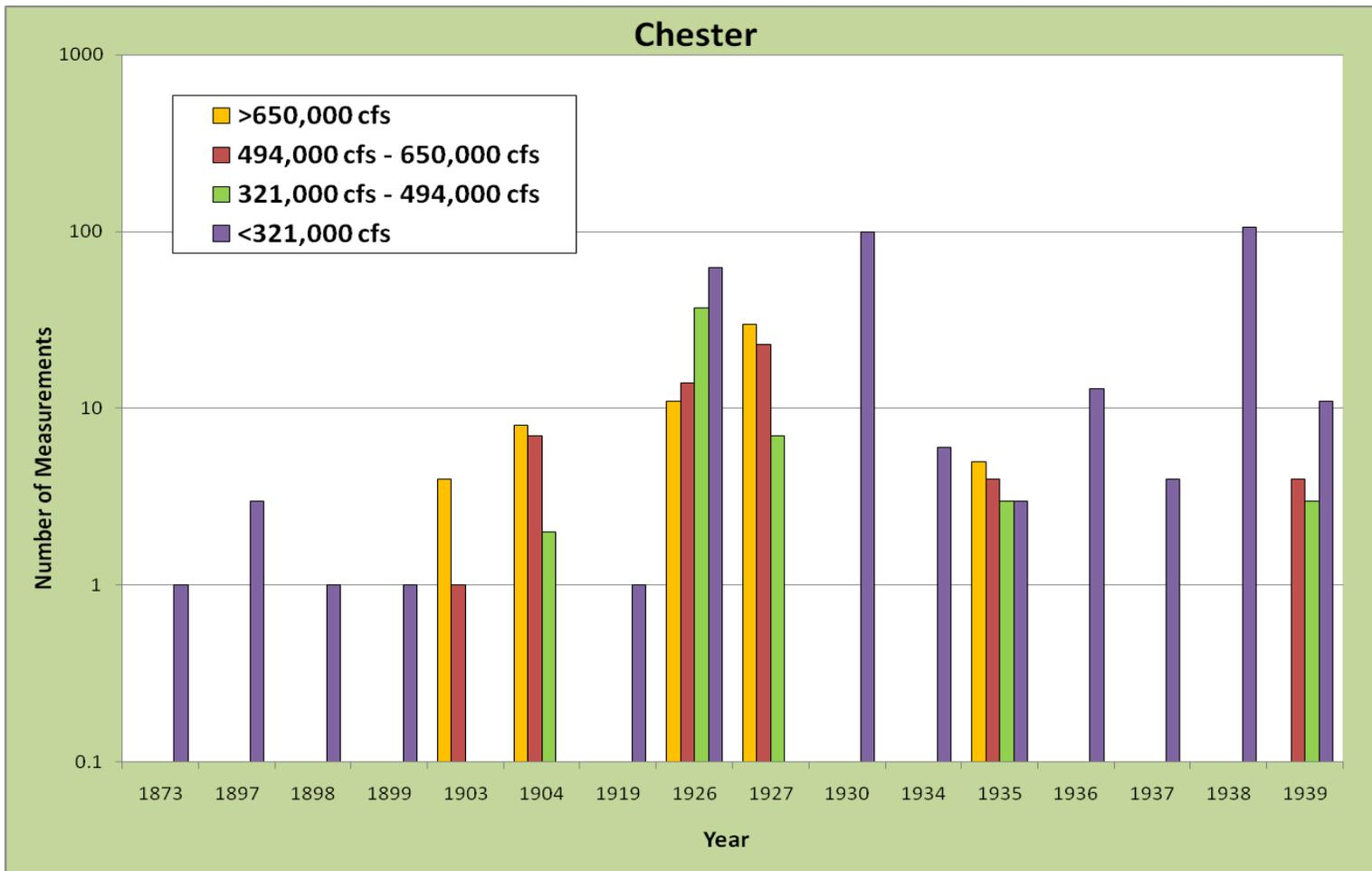
**Figure 4.5** The number of measurements made in four discharge ranges at Chester from 1873 to 1939.
