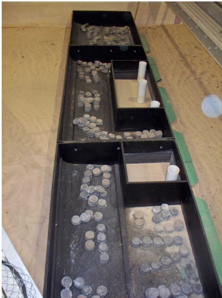
Figure 5 - Wooden raft used to simulate upstream ice
