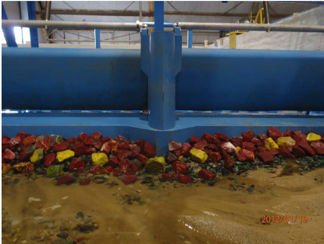
Figure 10 - 7 ft center gates, 20 ft ice raft draft
