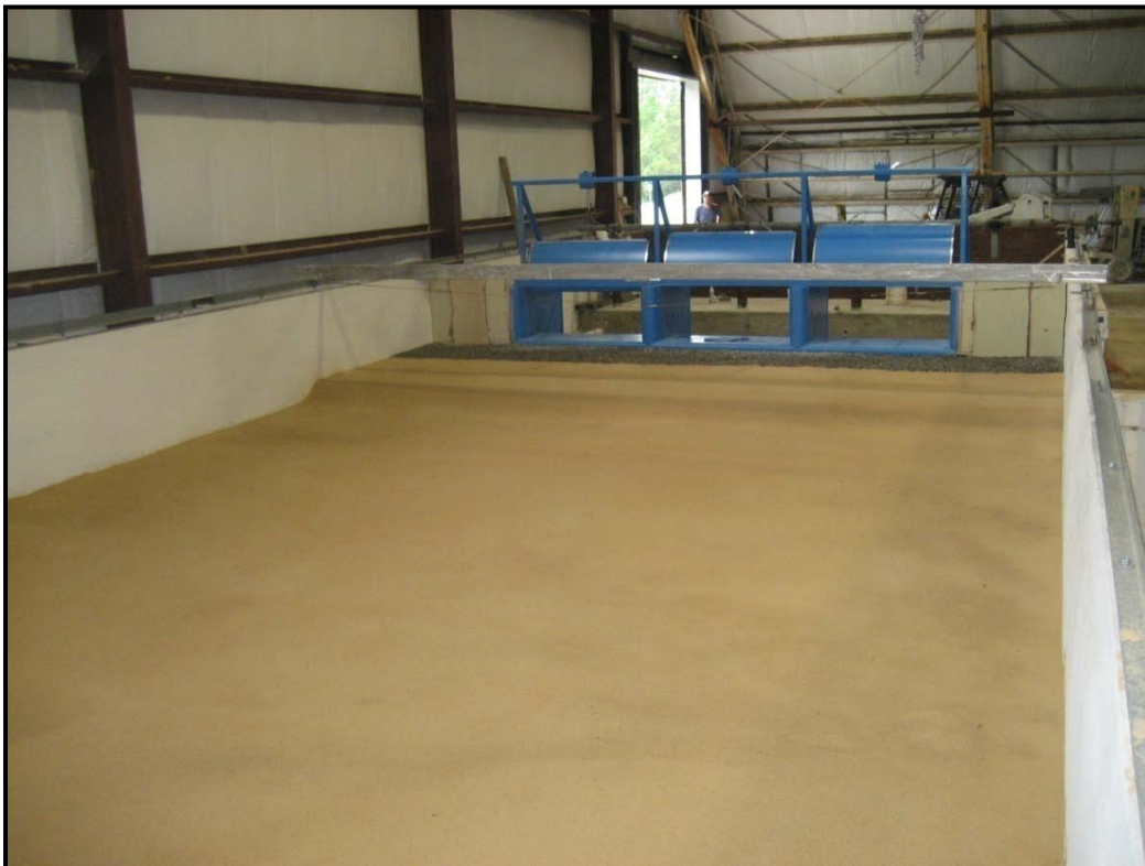
Figure 4 - The bed upstream of the model gate structure
