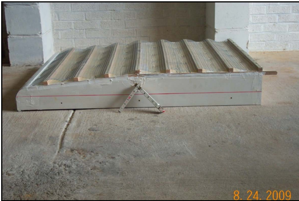
Figure 6 - Wooden raft used to simulate upstream ice
