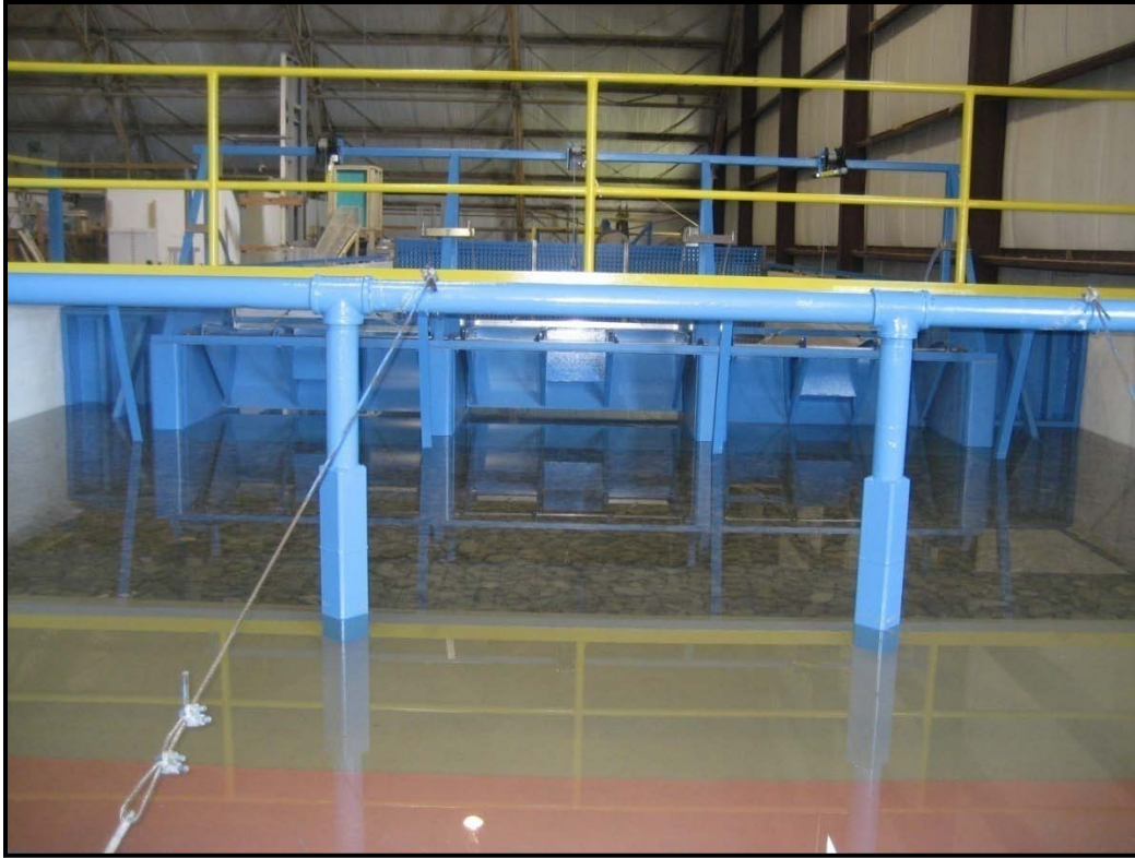
Figure 5 - The model gate structure and walkway viewed from downstream
