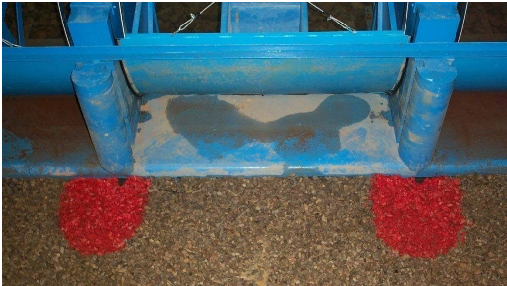
Figure 11 - The post-test 23 ft center gate opening, original stone, filter cloth, no ice
