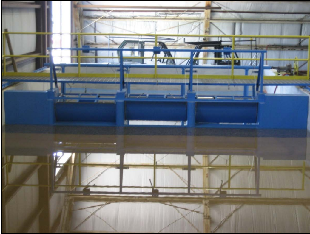
Figure 3 - The model gate structure and walkway viewed from upstream
