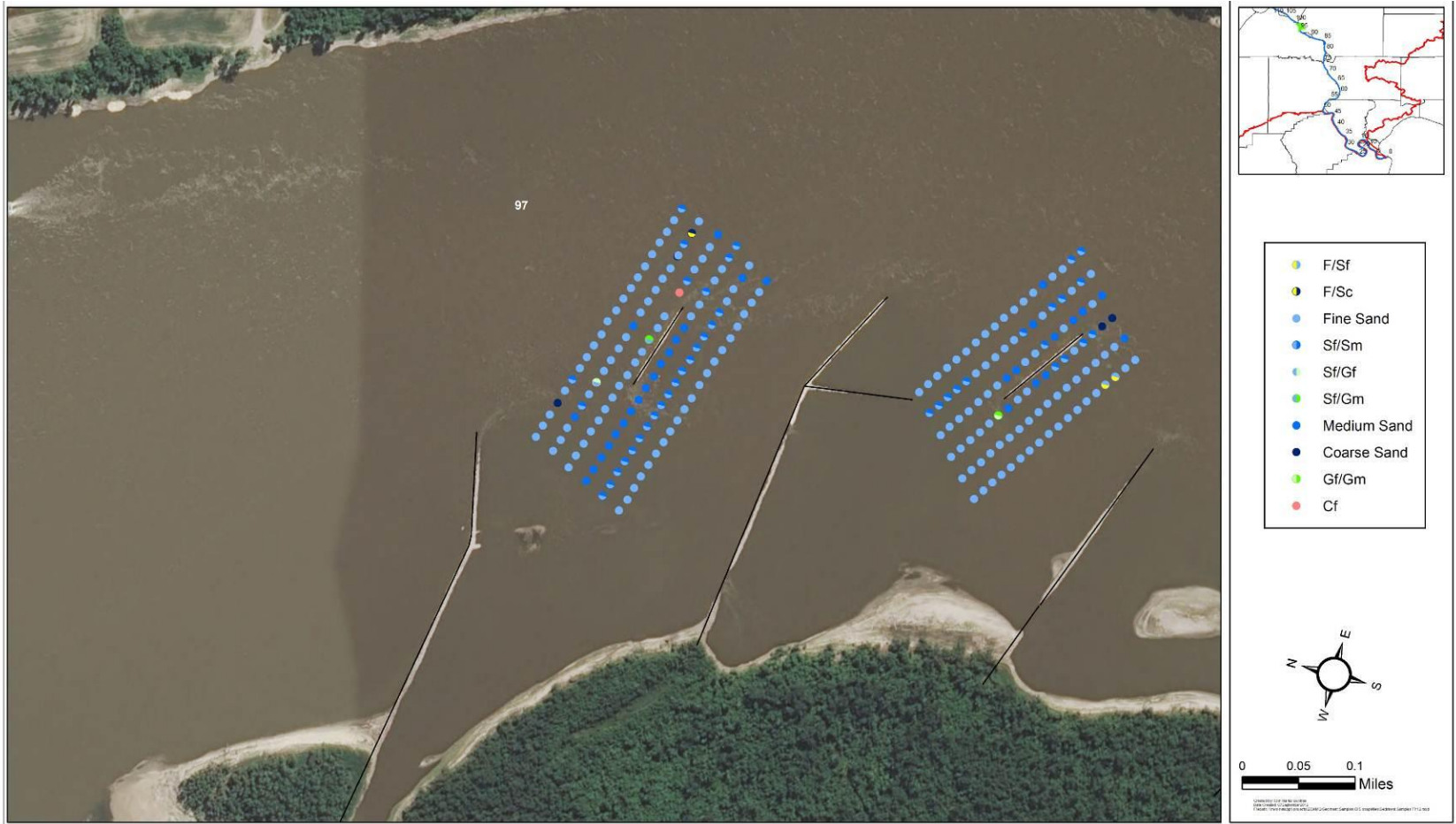
Exhibit 4. Sediment survey conducted on 16 & 17 August 2012 around the dike extensions at Mississippi River Mile 97. The first letter of abbreviations indicates F-fines, S-sand, G-gravel, and C-cobble classified into different size classes (2 nd letter) f-fine, s-small, m-medium, c-coarse, and l-large.
