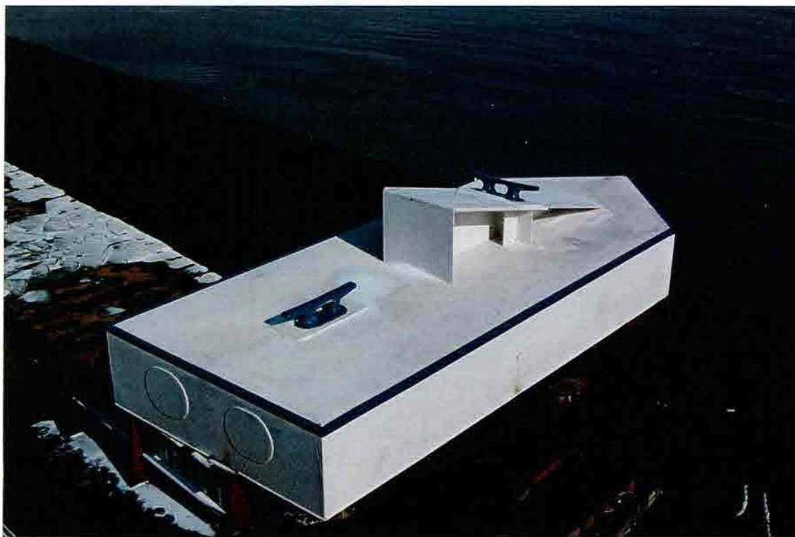
Prototype Buoy 30 Feet Long, 12 Feet Wide, Weight - 15 Tons
