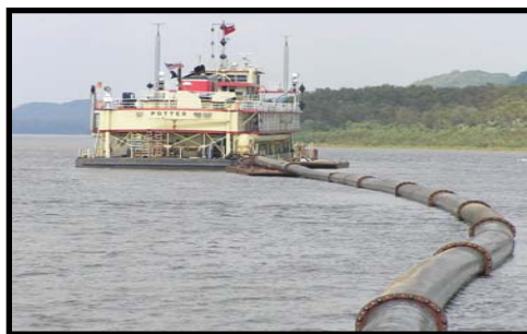
Figure 12: HDPE Pipe connected to Dredge Potter
