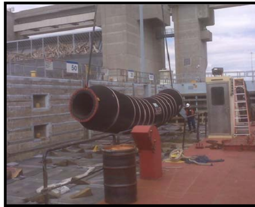
Figure 13: Flexible Floating Hose Section
