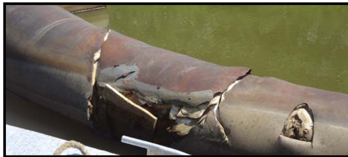
Figure 7: Deteriorated Flexible Floating Pipe
