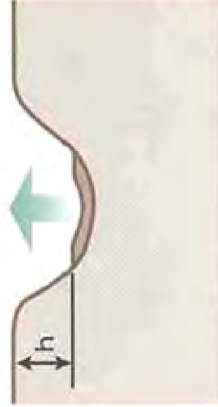
Class III. Degradation h < h_c
