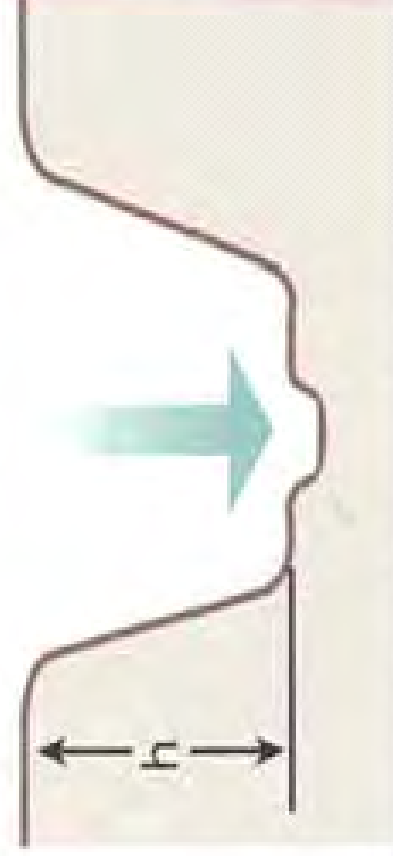
Class V. Aggradation and Widening h > h_c
