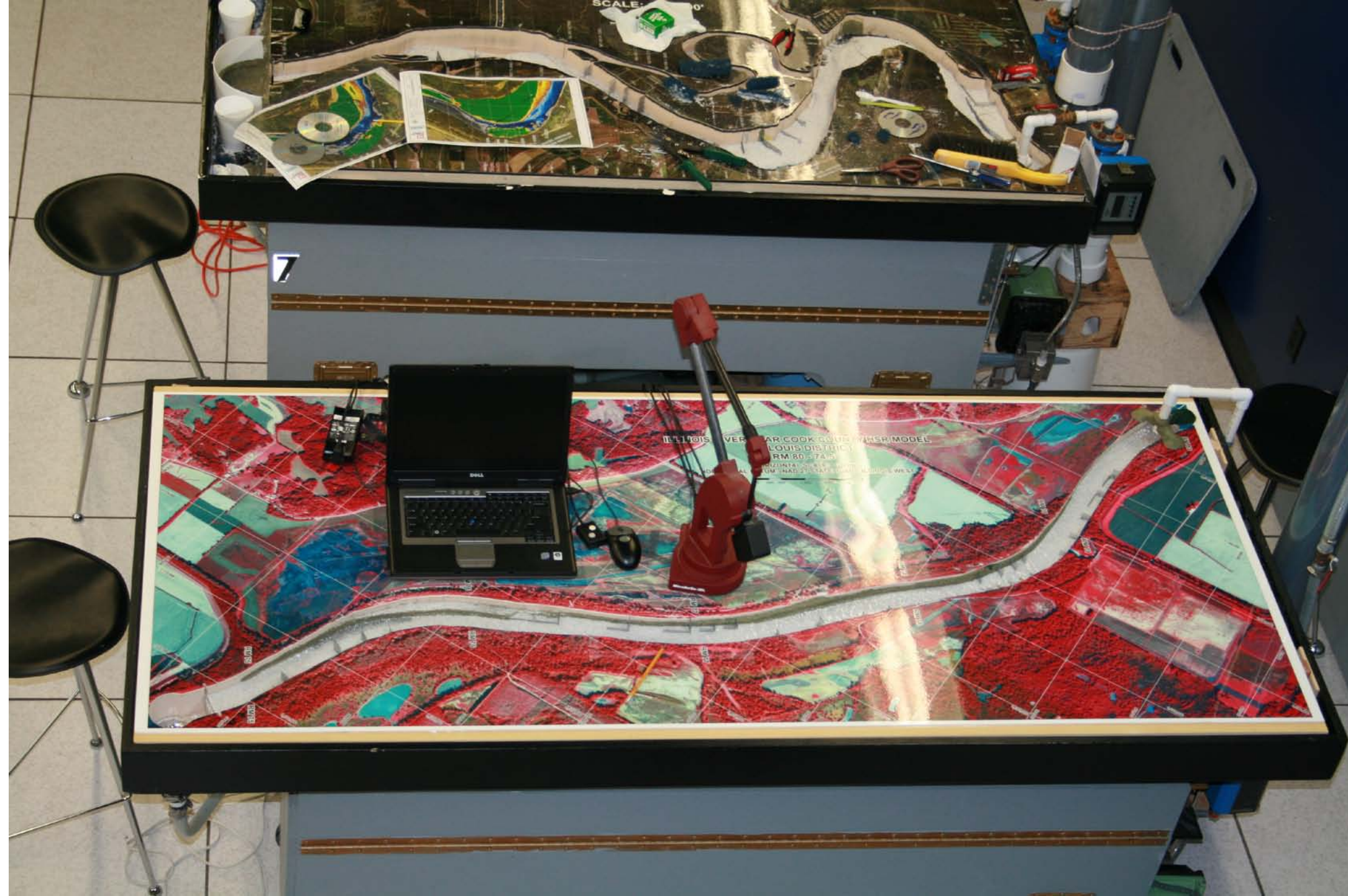
Illinois River Hydraulic Sediment Response Model
