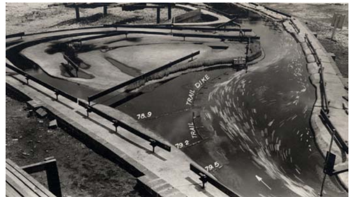
Railing system for large-scale coal bed models (U.S. Army Engineer Waterways Experiment 1937).
