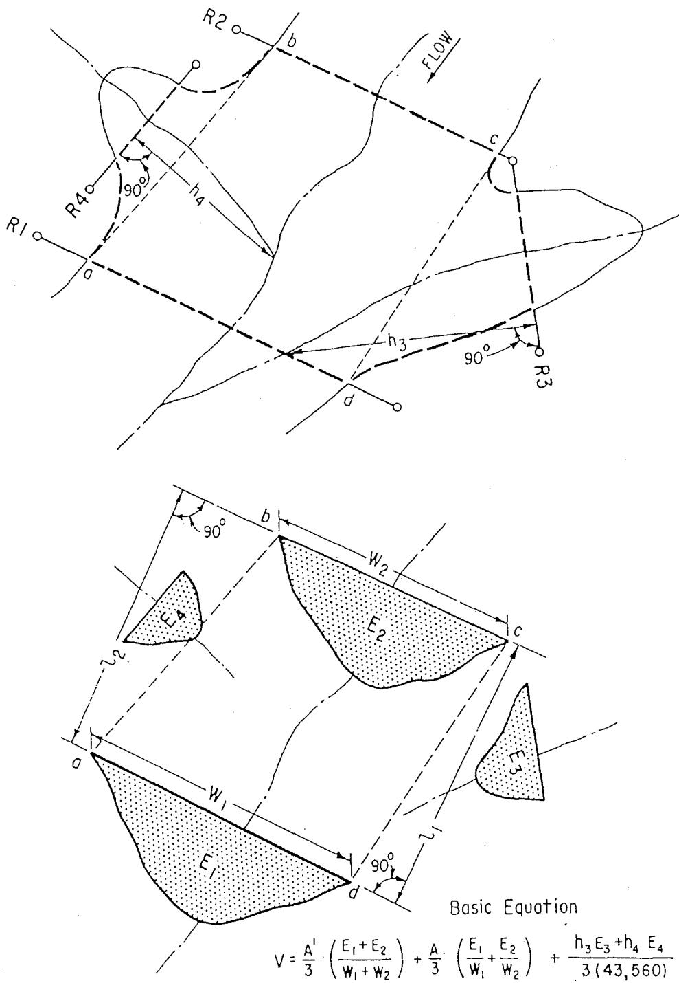
Figure 1. Terms of range-end formula for determining capacity of a reservoir. (Taken from ASCE M&R No. 54, "Sedimentation Engineering," V.A. Vanoni, Editor, 1975, pp. 378-379).
