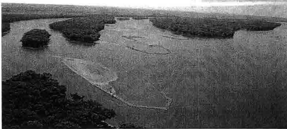
Figure B. Chevron dike field at Mississippi River mile 289. Note the dredge material islands formed behind each chevron.
