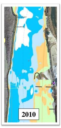
14. **Dike modifications at Big Muddy River confluence, RM 75.5(L) (Pallid Sturgeon - RPA 4, RPM 1; Least Tern RPM 1).** An extension of dike 75.3(L) was initiated in FY10 and was largely completed in FY11 (see image below; 2010 bathymetry does not reflect FY11 dike 75.3(L) impacts).
