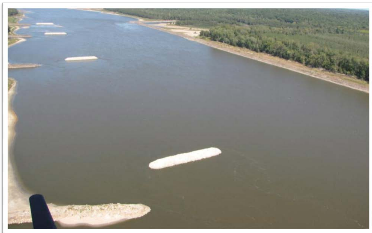
Thebes Reach offset dikes (RM 39R) during low-water fly-over September 2012 (river level -2.5 on St. Louis gage).
