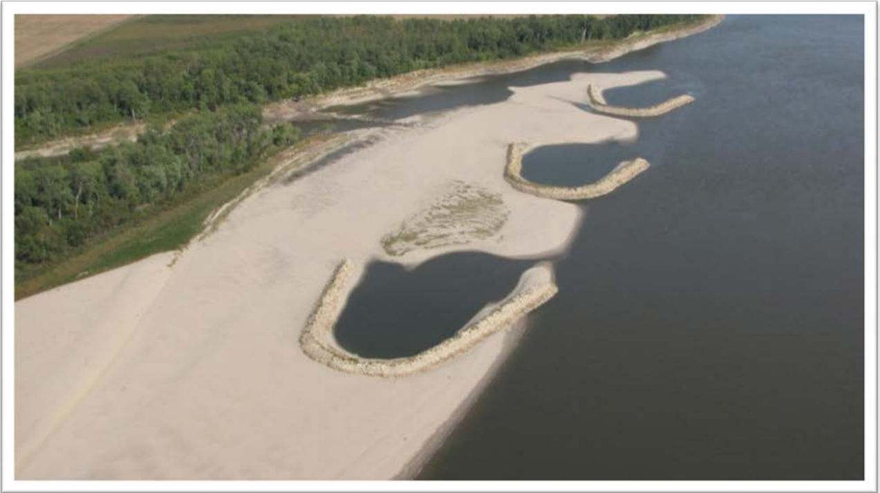
Liberty Chute chevrons (RM 100L) during low-water fly-over September 2012 (river level -2.5 on St. Louis gage).
