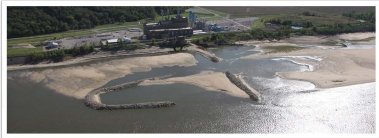
Grand Tower chevron and notched dike (RM 82L) during low-water fly-over September 2012 (river level -2.5 on St. Louis gage).
