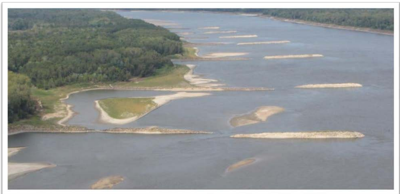
Devils Island offset dikes (RM 59-58R) during low-water fly-over September 2012 (river level -2.5 on St. Louis gage).
